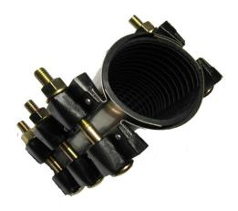
The REMCO 1286 Series Full Circumference Repair Clamp is designed to serve as a repair solution for pipe leakage. Depending on the size of the leak, this clamp can be used to repair holes, longitudinal and circumferential fractures, and
